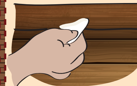
Use matching wood filler to conceal nail holes
