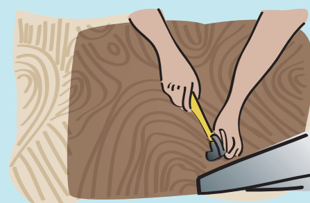
Install underlay material (Fix underlay to substrate)
