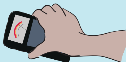
Measure moisture content of screed surface
